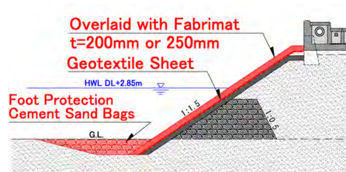
② : Overlay of existing revetment mat
