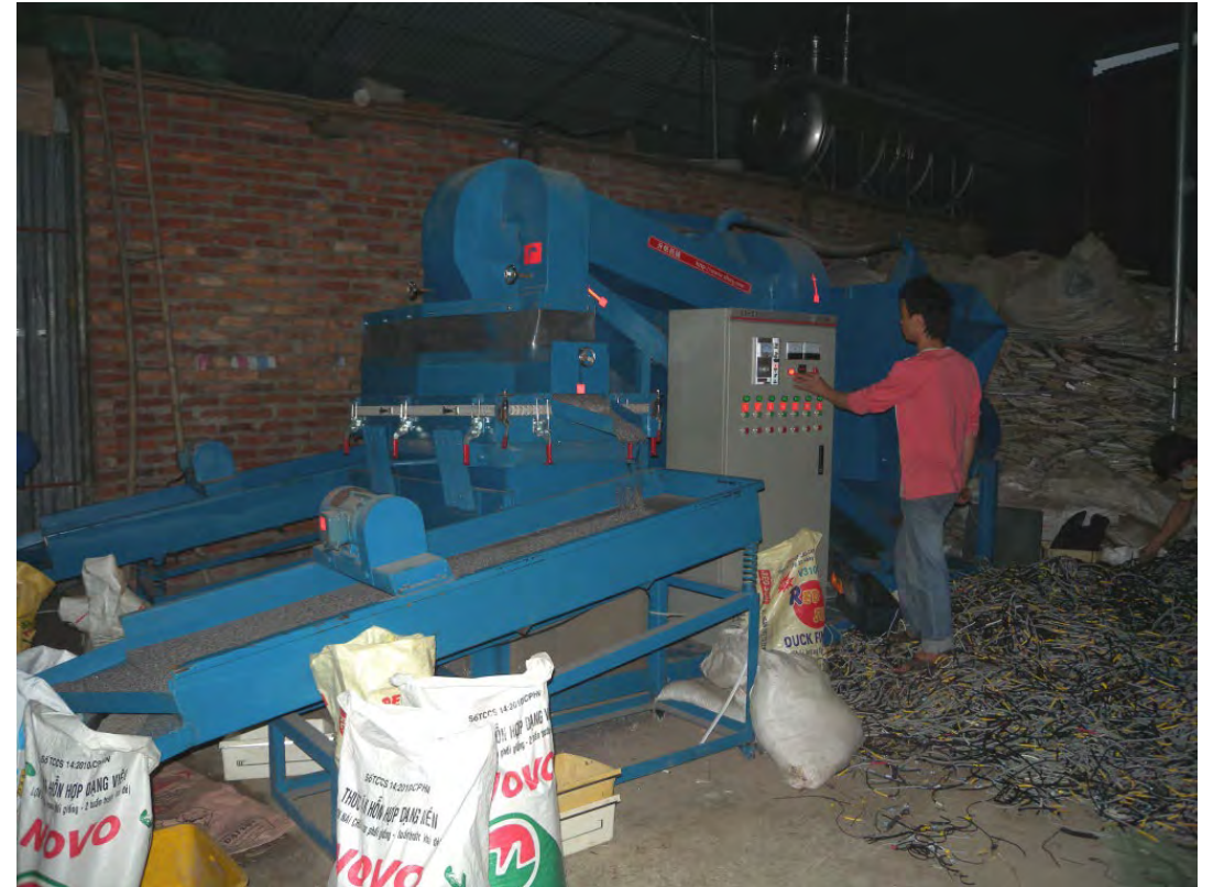
Machines to shred copper cables to separate plastics and copper, in Viet Nam , November 2012, Vietnam. Photo by M. Kojima
