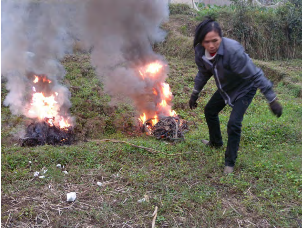
Open burning of copper cables, to remove plastics by use of fire, January 2011, Photo by M. Kojima, in suburb of Hanoi, Vietnam. 。
