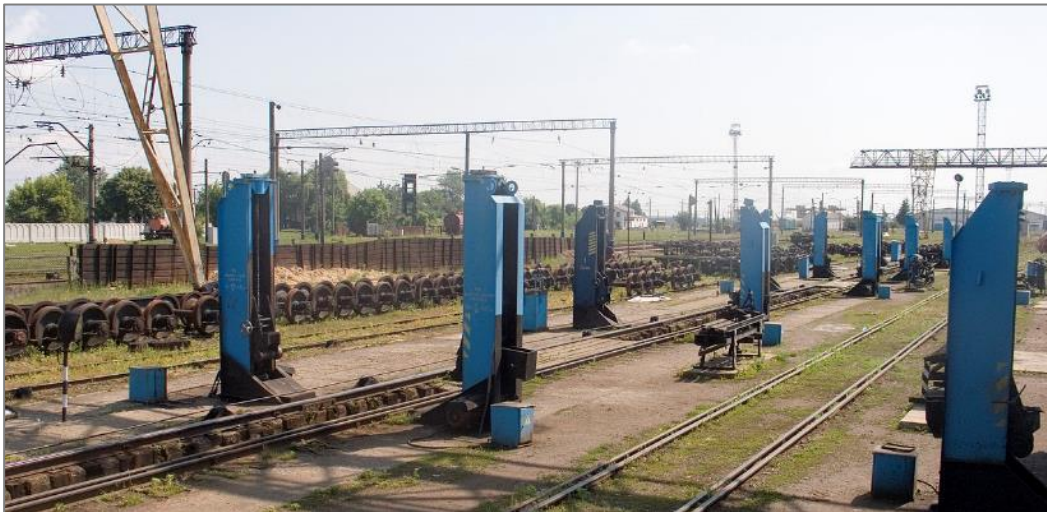
Figure 45: Bogie change station (Chop, Ukraine, between Russian gauge and standard gauge)
