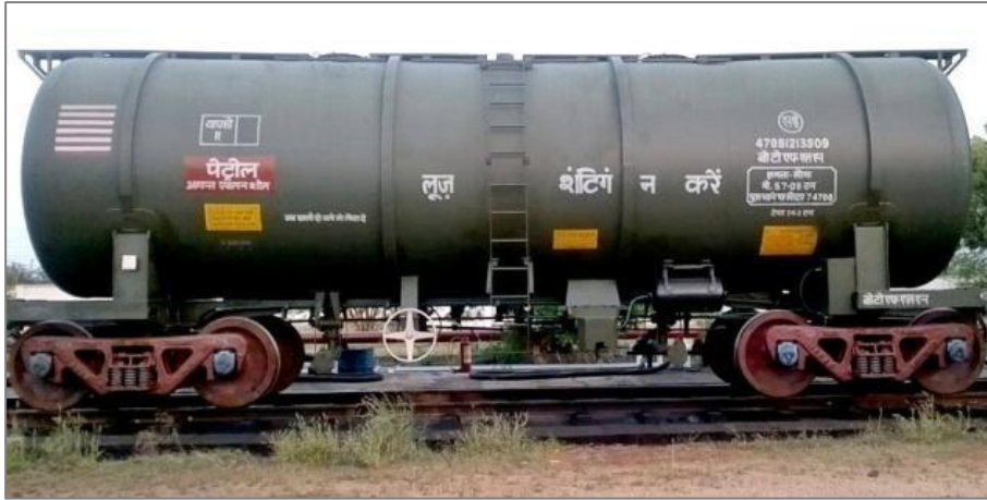
Figure 40: Example of freight wagon (tank wagon) (2/3) from IR
