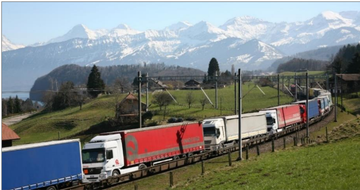
Figure 5: An image of the 'Rolling Road' in Switzerland (Source: RAIPin)
