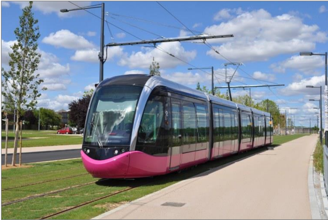
Figure 35: Example of a tramway (Dijon, France). This train can go in both directions without having to turn around.
