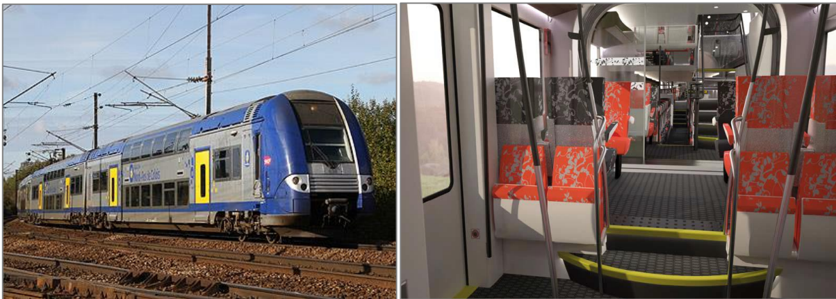
Figure 34:7 Example of a powered double deck rail car train. This train can go in both directions without turning around (France)
