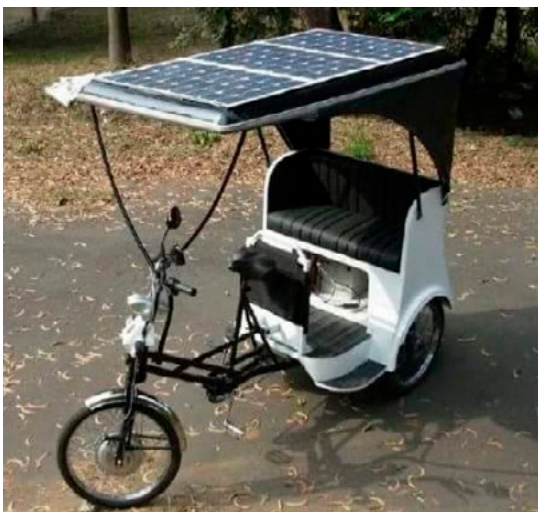
Fig. 37a, b: Tricycles with solar roof, being used as rickshaw. © SIKCO, 2015
