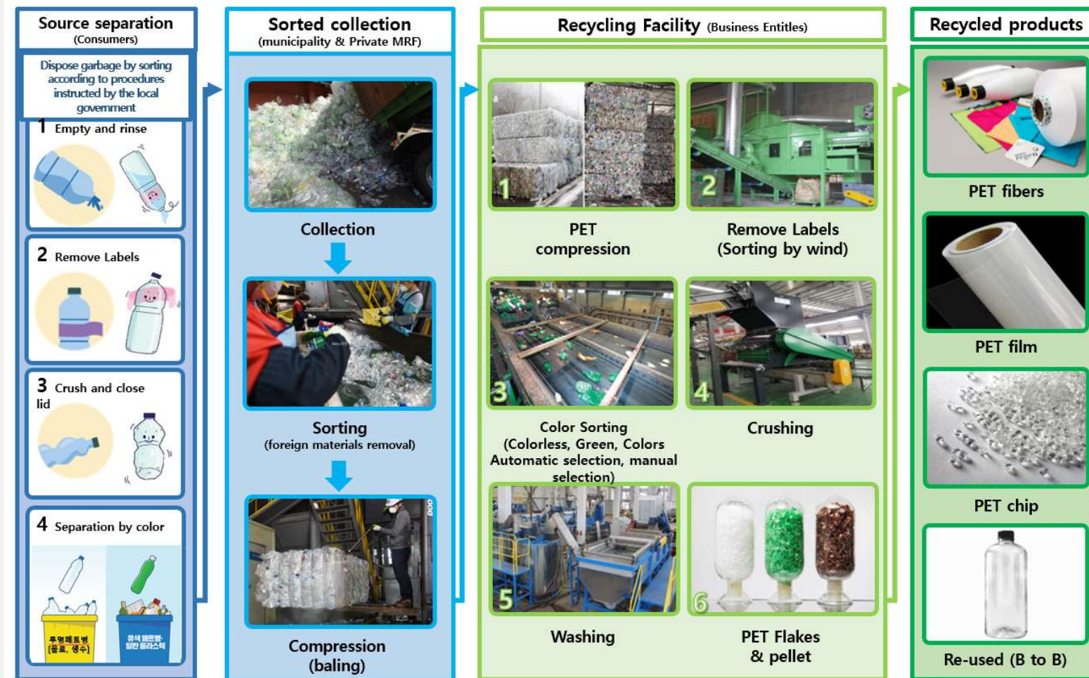
[Figure] PET bottle collection, sorting, and recycling flow from households in Korea
