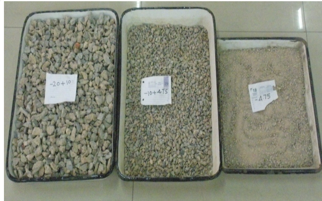
Recycled Concrete Aggregate
