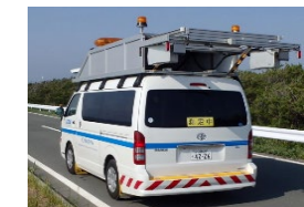
Pavement damage detection by 3D laser sensor
