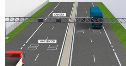
The system is able to weigh a vehicle while in motion automatically and continuously. Therefore, it can provide accurate vehicle weight information to enforcement and efficient enforcement implementation.
