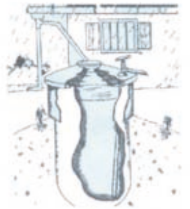
Partially underground tank
