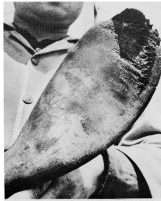
Corroded boat propeller in the toxic sea
