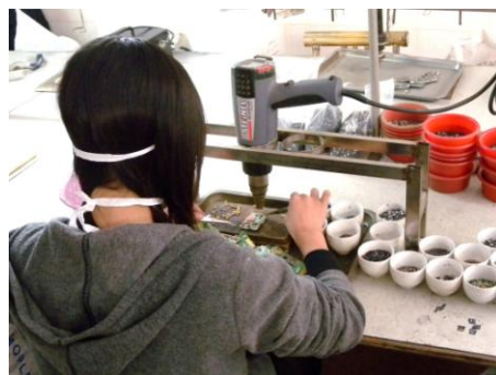
Removing IC tips from printed circuit board for mobile phone, using equipment similar to hair dryer. (December 2009, Guiyu, China)
