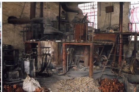
Producing copper cable from waste copper without refinery process. (August, 2002, China)
