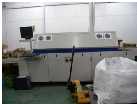
A machine removing IC tips from Printed Circuit Board (December 2011, Hong Kong)
