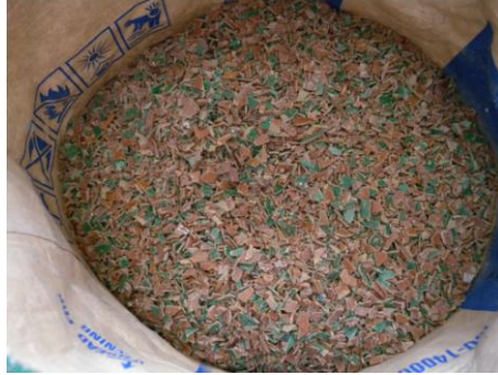
Crushed printed circuit board, which is sent to Cement industry. (September 2010, Indonesia)
