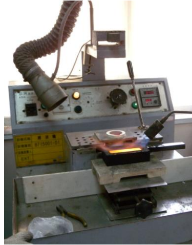
Gold recovery using cyanide and heat, in e-waste recycling factory in Taiwan.
