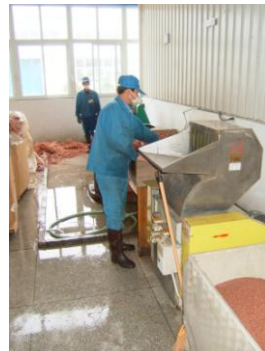
Nagget system to separate copper and plastics. (Dec, 2004)
