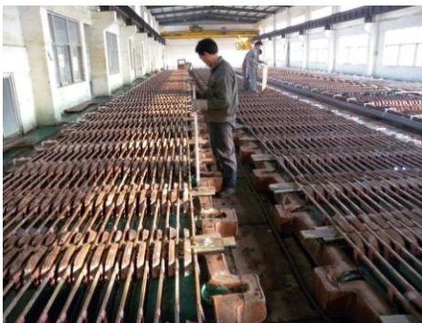
Copper refining process using electrolysis , December 2009, Guiyu, China
