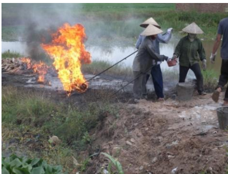
Open burning of plastic-coated wire to extract copper. Vietnam, August 2009.
