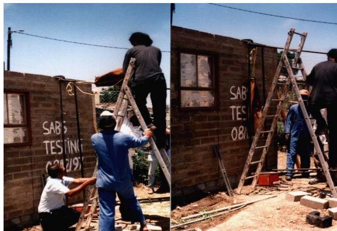
Heavy load impact test
