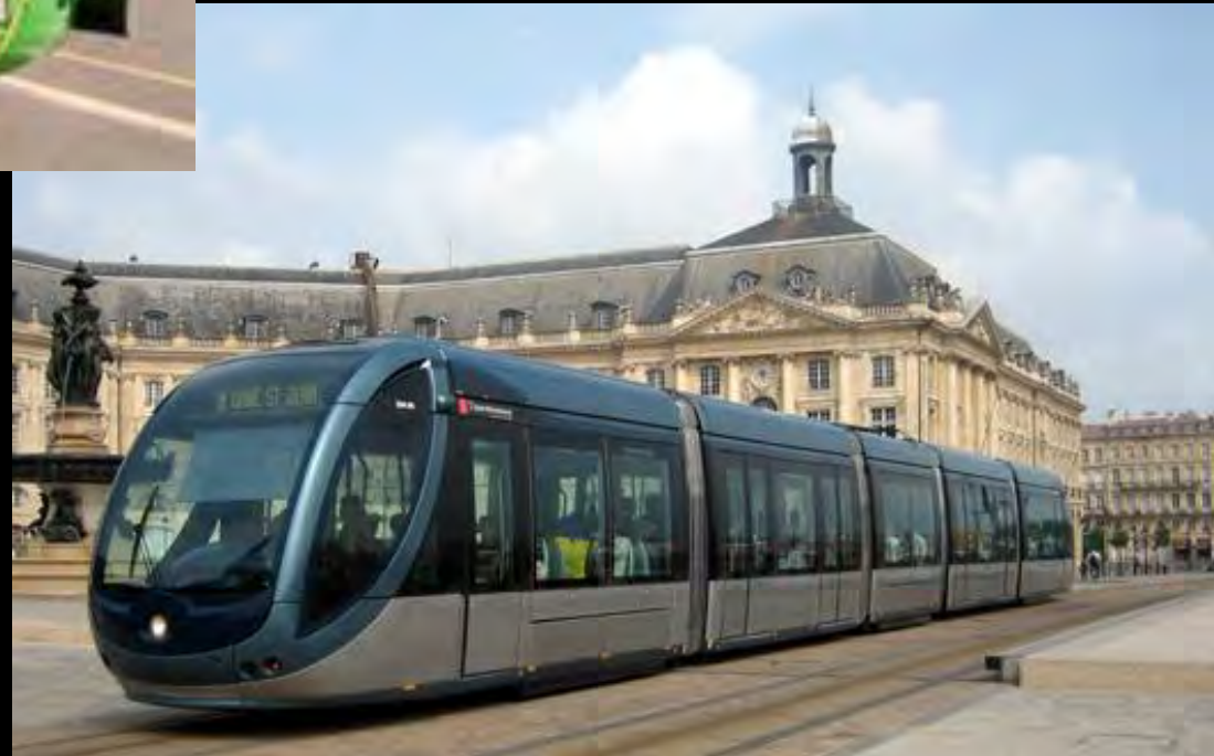
Alstom battery-powered light rail in Bordeaux
