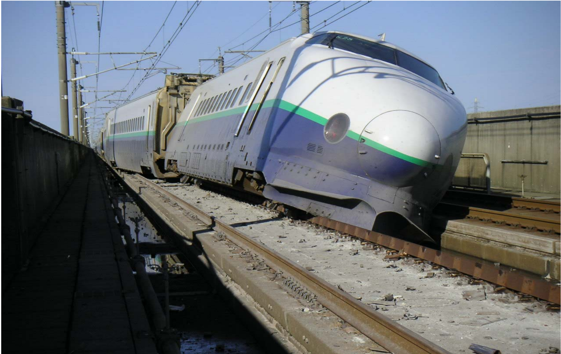
Derailed Shinkansen cars by Niigata Prefecture Chuetsu Earthquake in October 2004
