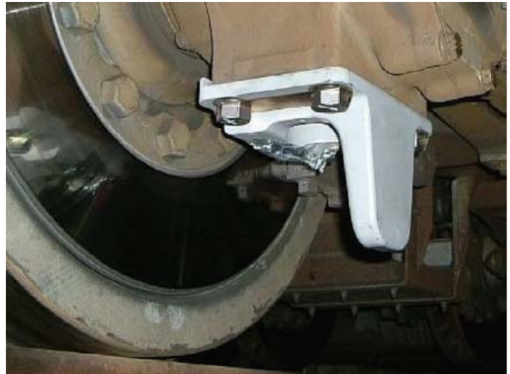
L-shaped guide to prevent deviation from rails
