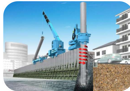
Low-noise piling system for disaster-resistant infrastructure
