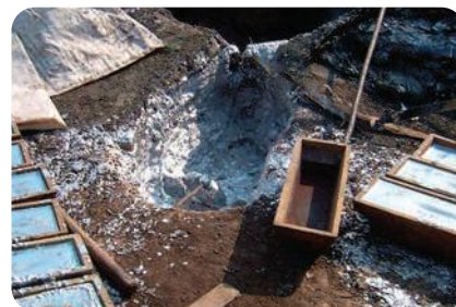
Smelting lead and making ingots. Soil was contaminated with lead.
