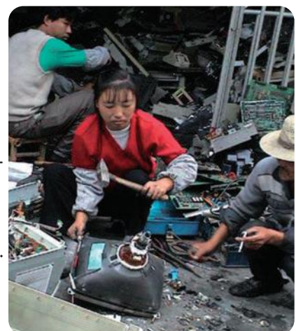
Unprotected dismantler cracking the yoke of a Cathode Ray Tube (CRT) screen. Source: International Institute for Sustainable Development (IISD)(2008).
