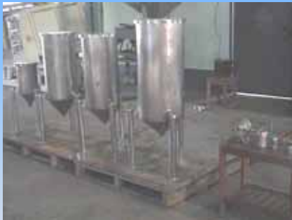
Pilot Plant of Biodiesel Processor 60 litre/day
