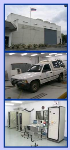
Testing on Chassis Dynamometer
