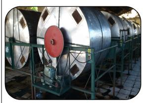
Photo 5 The MRF at Sta. Cruz Market is equipped with circular composting bins utilizing the patented "Happy Soil System Technology."
