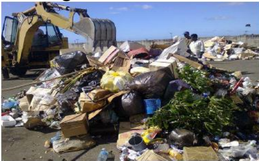
Mechanical Quartering of wastes
