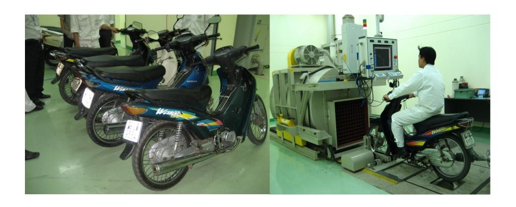
Emission Test before and after maintenance & repair
