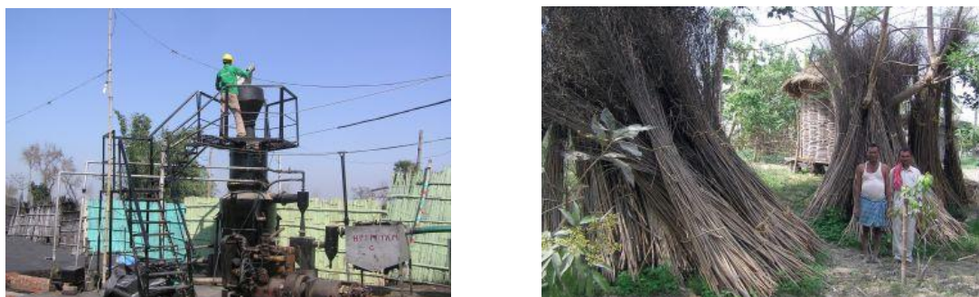
Figure 5. Filling gasifier plant with rice husk, Tamkuha and Dhaincha is the main fuel for SRE's gasifier plant, in Bihar, India (Source: http://www.ashden.org/winners/husk11 02.10.2016)
