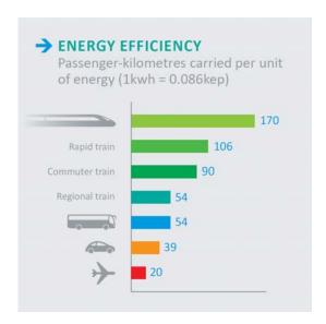
Comparison of energy efficiency for high speed rail and other transport modes
