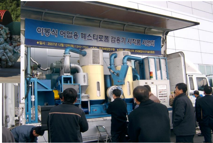
Collected buoy melting facility for recycling
