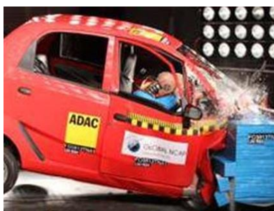
Figure 22 Example of result of NCAP frontal test on vehicle sold in Indian market [65]
