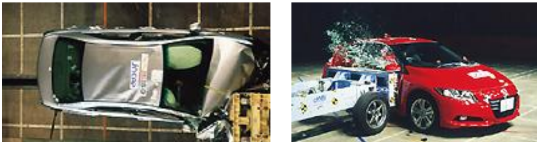
Figure 21 Examples of crash tests in JNCAP, Japanese NCAP – frontal partial overlap test (left), side impact test (right) [64]
