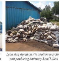
Lead slag stored on site battery recycling unit producing Antimony-Lead billets
