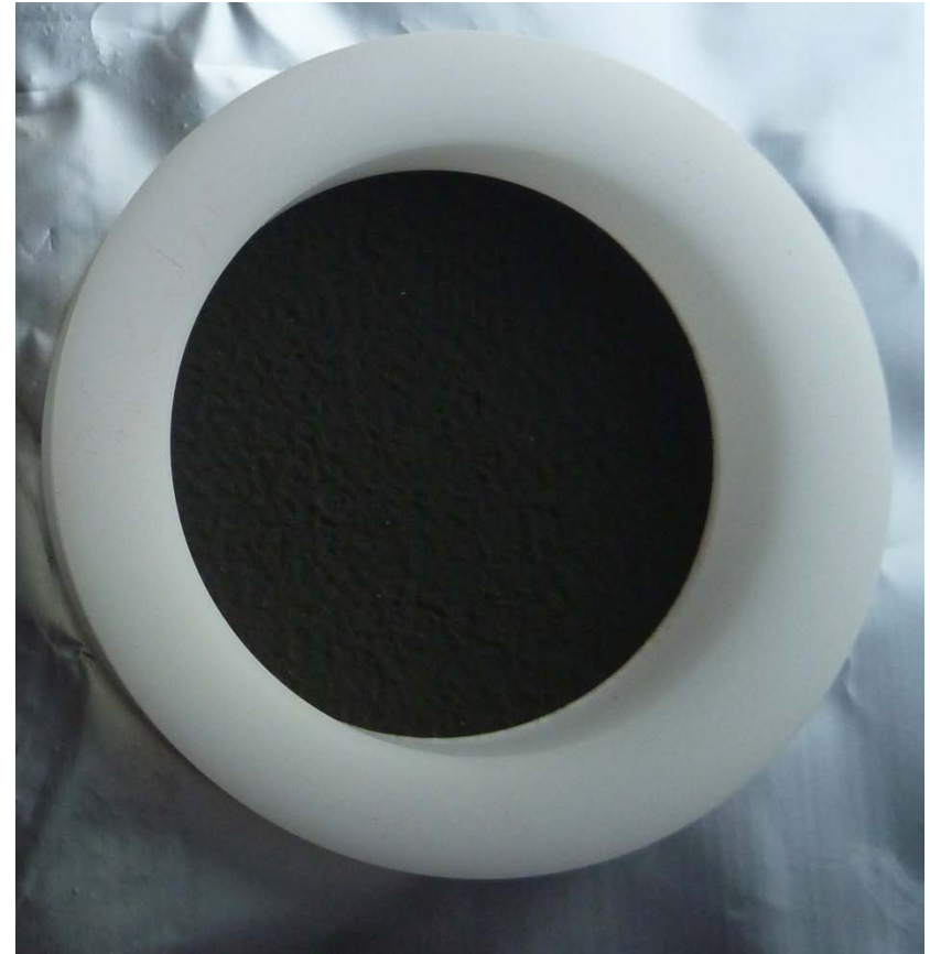
The same filter, after 24 hours of sampling Kathmandu Valley air
