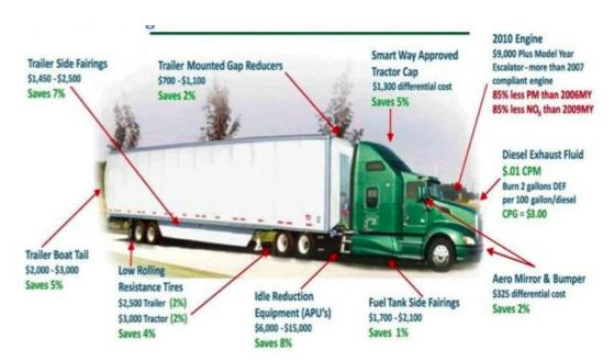
Figure 8: Truck technologies for greener freight (Source: Polovick 2011)
