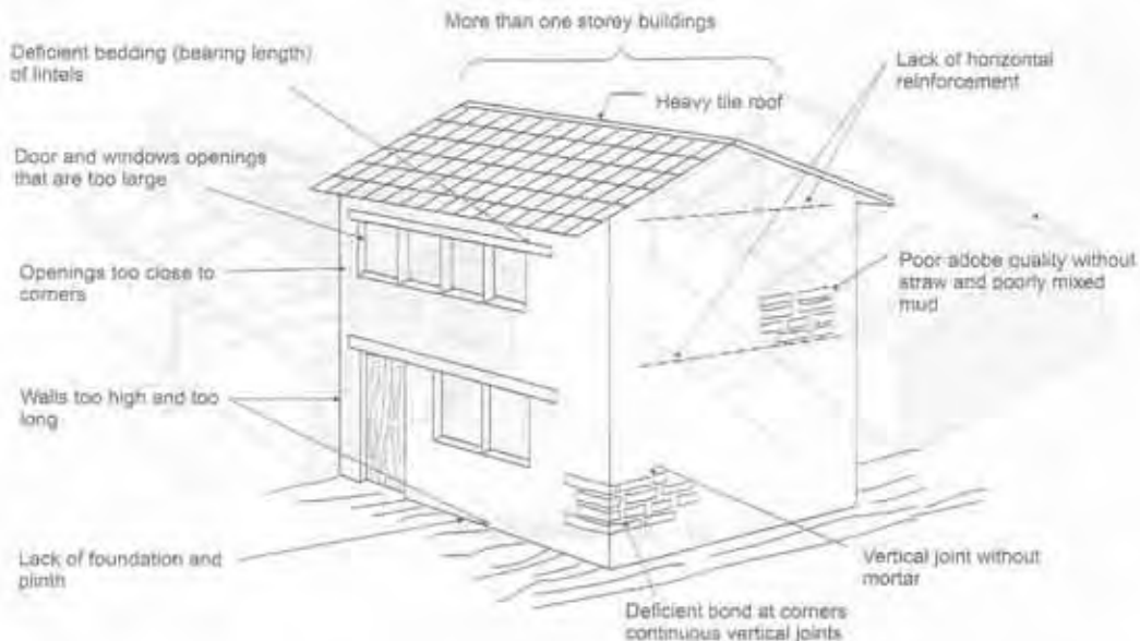
Fig. 2E Summary of main causes of failure
