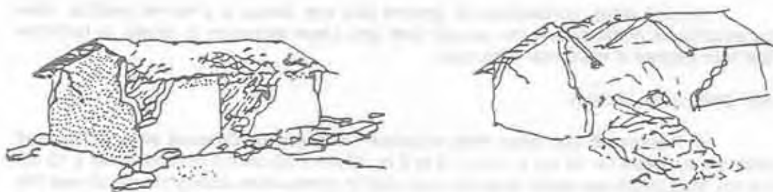
a) Corner Failure and out of Plane Collapse of Walls
