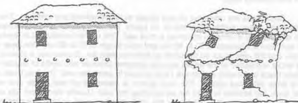
b) Two Storey House Damage/Collapse
