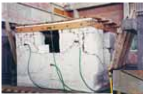
Full scale model 1,0g pga. Roof did not fall
