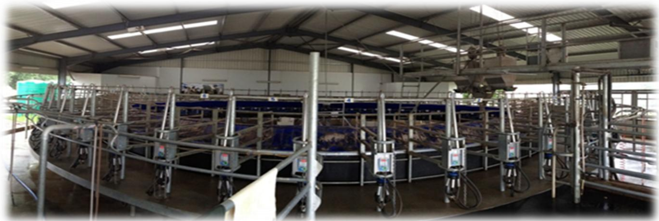
Advanced Rotary Dairy system with cow retention time of approx. 11 minutes
