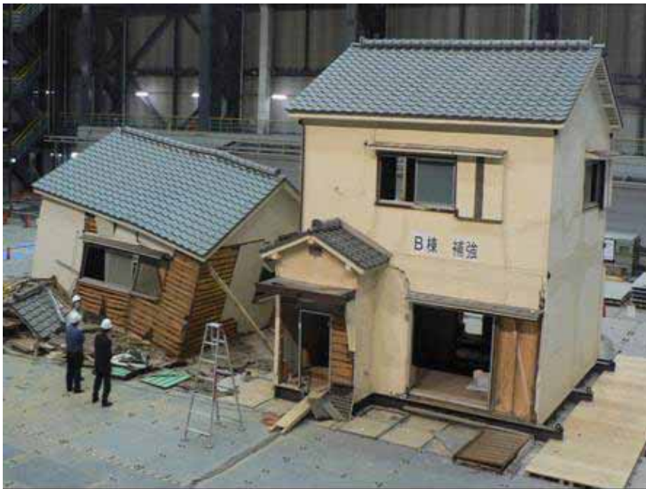
Photo 4: Shaking table tests on conventional wooden houses at E-defense (21 Nov 2005)
