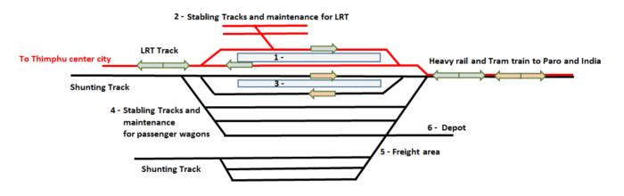
Figure 49: Example of configuration for Thimphu Railway Main Station
