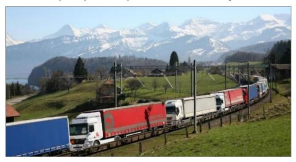
Figure 5: An image of the 'Rolling Road' in Switzerland (Source: RAlpin)
