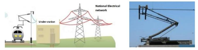
**Figure 68**: Electrical power supply from National network to catenary **Figure 69**: Pantograph Amongst the advantages of electrical traction are that it allows a higher rated power supply to be provided to the rolling stock and local pollution and maintenance costs are reduced. Electric traction is not dependent on supplies of fossil fuel.
