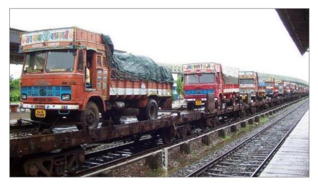
Figure 6: An image of the 'Roll-on Roll-off' train in India.
