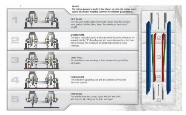
Figure 44: Talgo (change of gauge) process.
