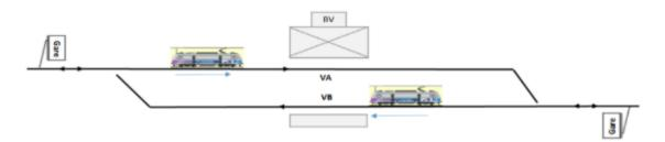
Figure 70: Left hand operating loop
