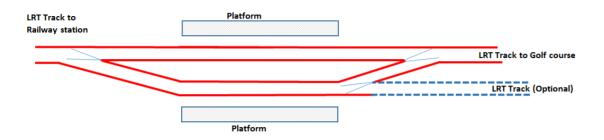
Figure 50: Example of configuration for Thimphu Urban Station (on this schematic, the track is presented with the two rails)
