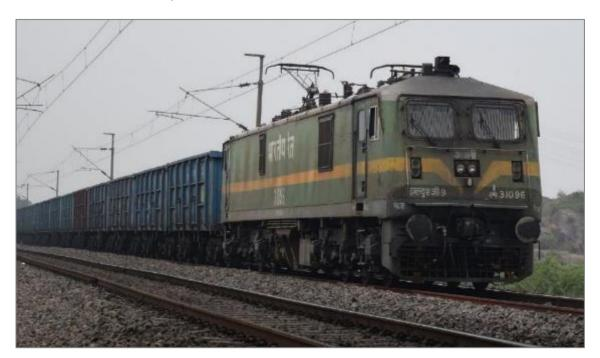
Figure 38: WAG9 locomotive (IR)
