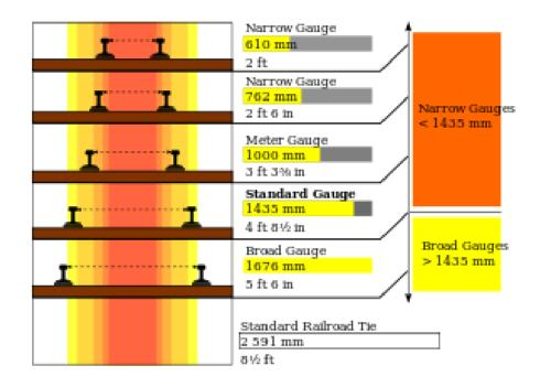
Figure 43: Examples of different categories of railway gauges
