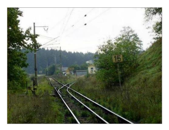
Figure 46: Two-gauge railway (metric gauge and standard) in Jindřichův Hradec (Czech Republic)
