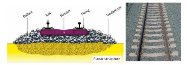
Figure 65: Structure of a track
