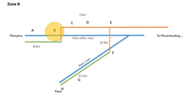
In this area, the line must pass over the river to move to the other of side of the valley, however, there are existing buildings and civil infrastructure that would need to be removed in order to make way for the new rail line.
