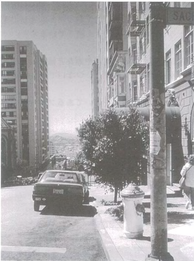
■ 1-29 Red cap, a fireplug located on the upper zone. (S.F.)
