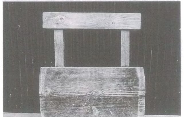
■ 1-58 Wooden adjustment board, which can easily increase or decrease the volume of water.
