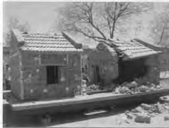
Stone with cement mortar -improved (left) vs. normal (right) model-
