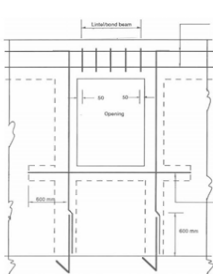
Figure 56: Reinforcement details around openings in walls
