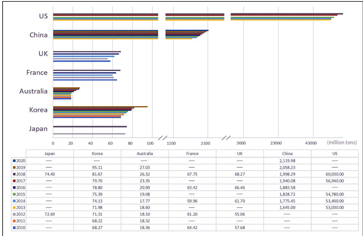
Figure 3.2.4-2: CDW Quantification and generation annual amount of some countries in Asia and the Pacific (ABD, 2016; DCCEEW Australia, 2020; Deloitte, 2015a; EPA US, 2018; MOEJ, 2018; Research and Markets Globe Newswire, 2021).
