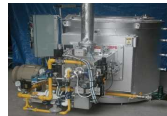
Regenerative Burners in industries, Toyotsu Machinery, Indonesia
