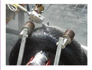
Water jet technology is an emerging and eco-friendly method for producing crumb rubber, offering a sustainable alternative to conventional mechanical and cryogenic grinding techniques. This technology involves using high-pressure water jets to break down waste tyres into fine rubber particles without generating excessive heat or requiring chemical treatments.
