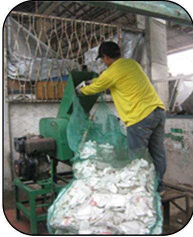
Photo 9 Waste materials are fed into the Styro / Plastic Densifier and Grinding Machine that is operated by the City Government.
