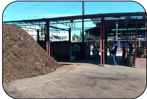
Photo 6 The pile of composted material will be sun dried before it will be sorted, packaged, and marketed.
