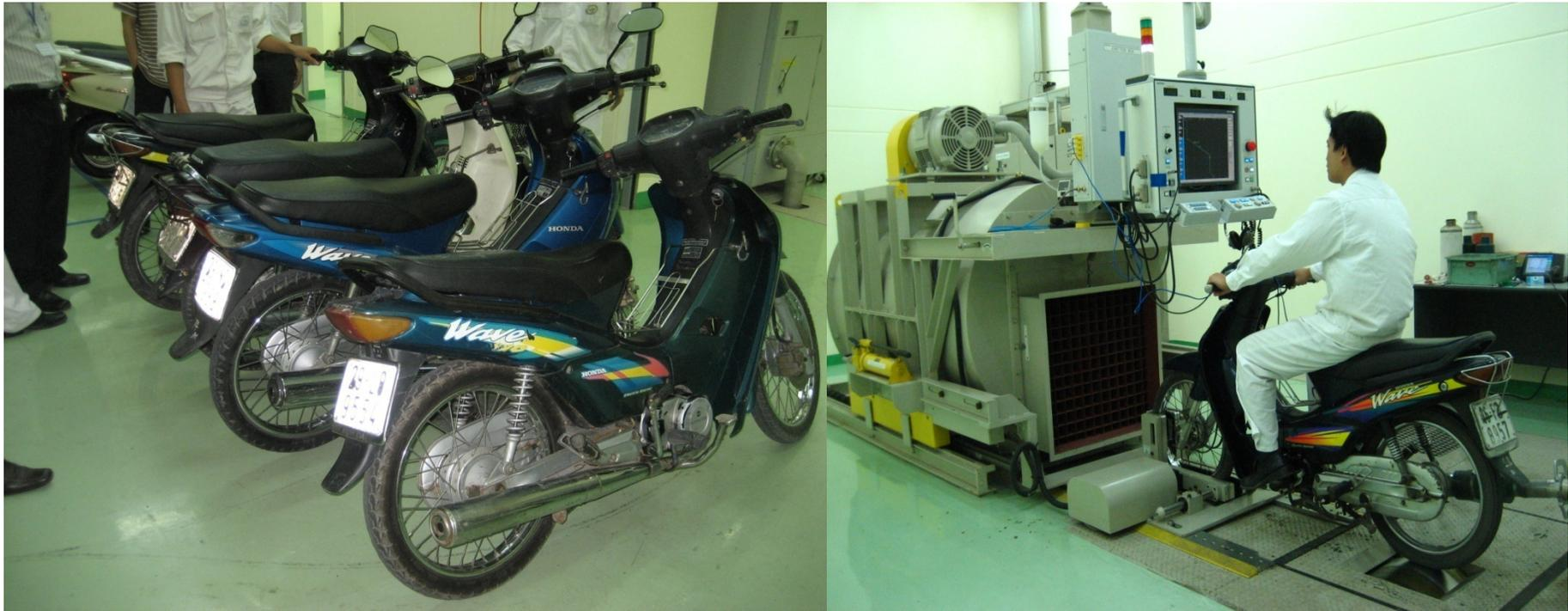
**Emission Test before and after maintenance & repair**
