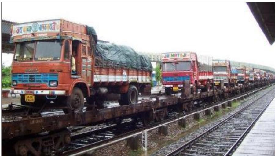
Figure 42: An image of the 'Roll-on Roll-off' train in India
