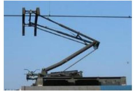
**Figure 68:** Electrical power supply from National network to catenary      **Figure 69:** Pantograph
