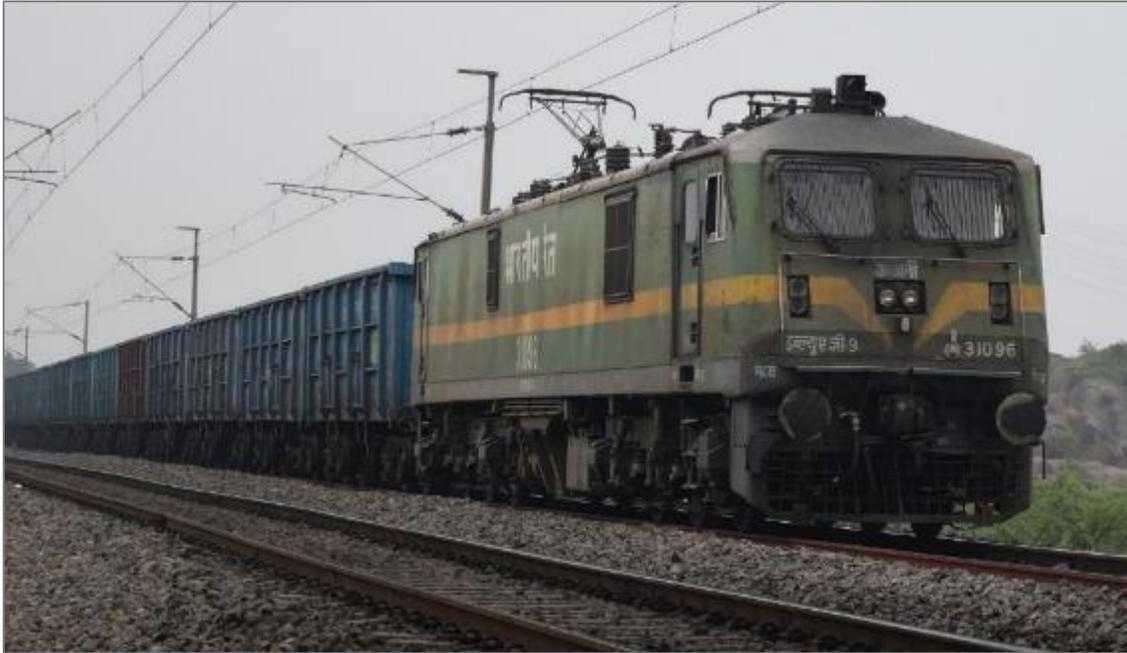
**Figure 38:** WAG9 locomotive (IR)
